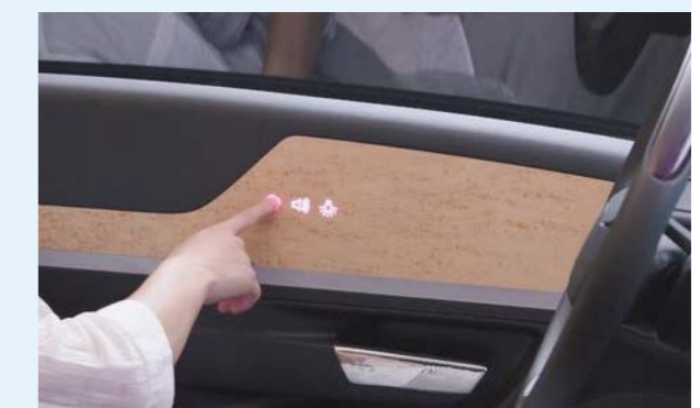
Touch switches that light up during operation
