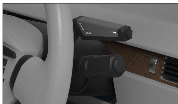
▲ Image of in-vehicle electric parking brake
